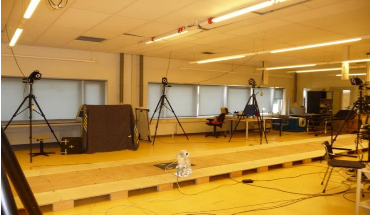
Figure 10: An overview of the movement lab, the place where Gait Analysis has been adopted of the Nao H25. The Nao walks over a 12-meter-long walkway with incorporated force platform in the middle while the movement of the markers can be recorded by the different cameras surrounding the walkway.
