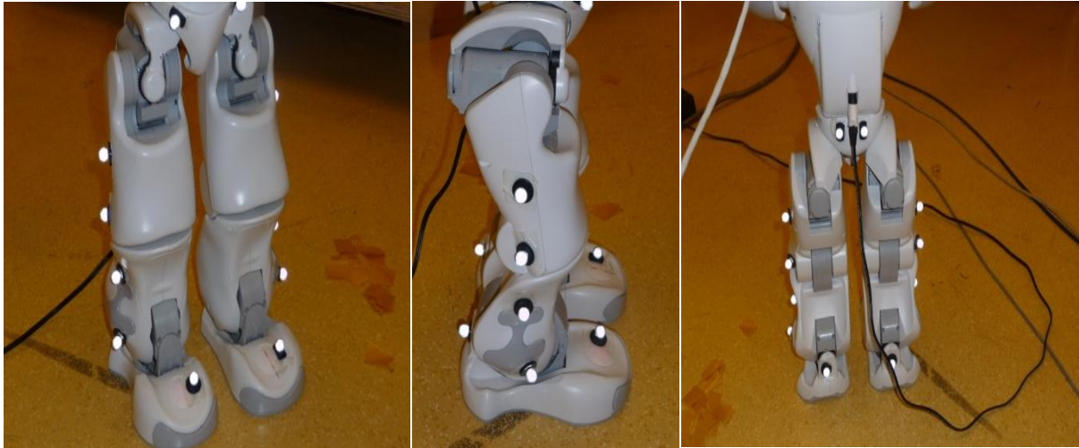
Figure 11abc: Sixteen different markers were placed on the different DOFs of the Nao H25.
